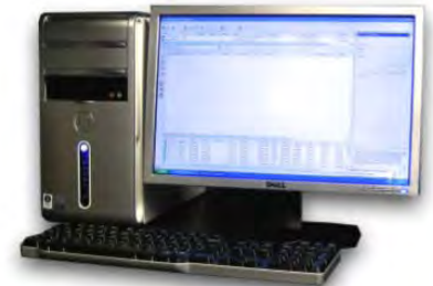
Onyx Production House RIP and printer server to allow seven-channel control of printer
